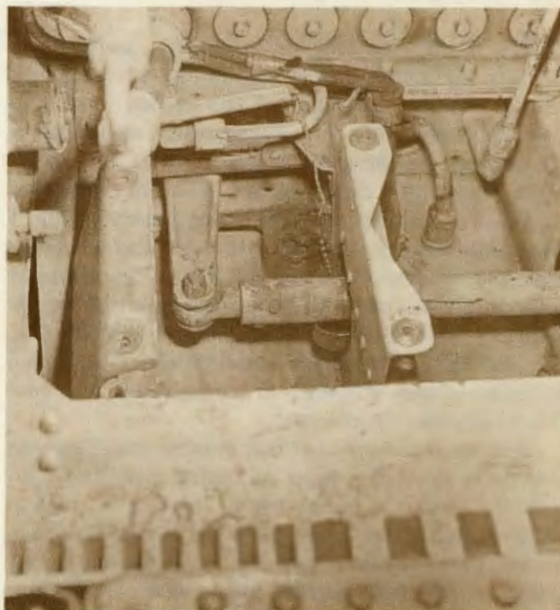
3. Jammed Aileron Control Rod (Switch Panel Removed)
