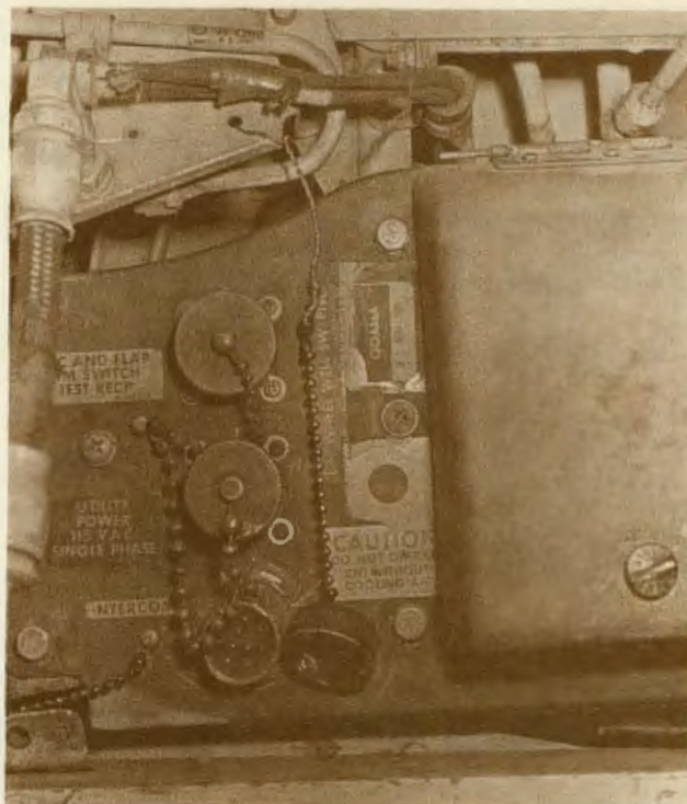
2. Illustration of Jury-Rigged Dust Cover Chain
